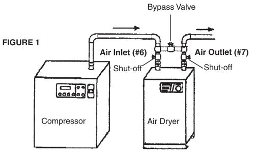
**Note to professional installer:** The shut-offs (not included) for both the air inlet and air outlet, must be plumbed below the horizontal piping containing the bypass valve. See **FIG-URE 1**.
